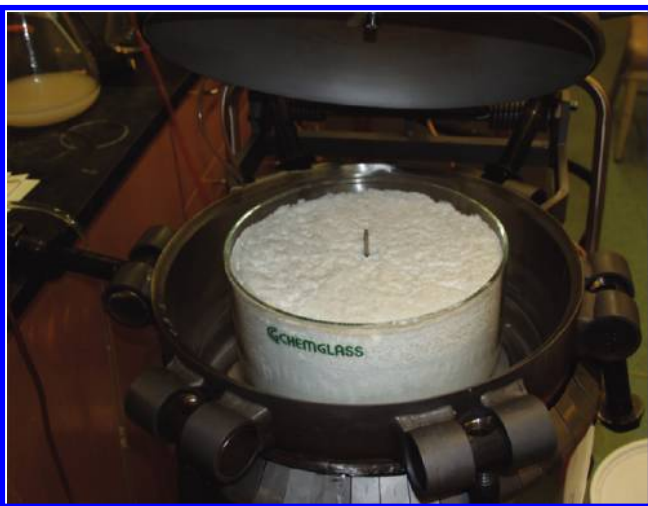
Figure 8. The sodium salt of 7 precipitates during the course of the reaction. Upon completion, the solvent is ejected, rapidly cooling the product which remains in the vessel as a spongy solid that is easily isolated by filtration.
