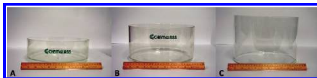
Figure 2. Interchangeable reaction flasks of (a) 5-L, (b) 9-L, and (c) 13-L capacity with working volumes of 2–4 L, 4–8 L, and 7–12 L, respectively.
